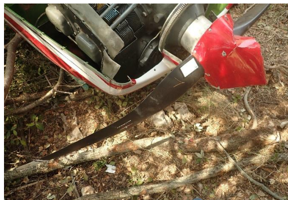
Picture 9 – Bending of propeller arm no. 2
