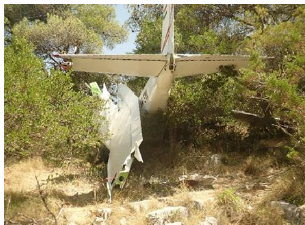
Picture 3 – Bent left wing along the fuselage
