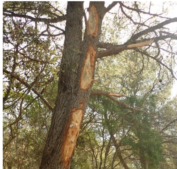
Picture 17 – Traces of the impact of the rotating propeller to the tree
