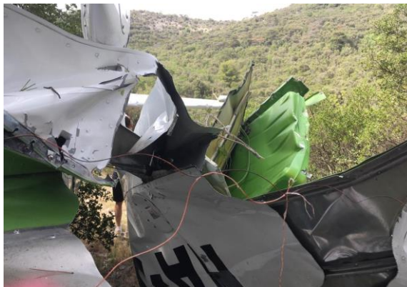
Picture 14 – Left wing fuel tank
