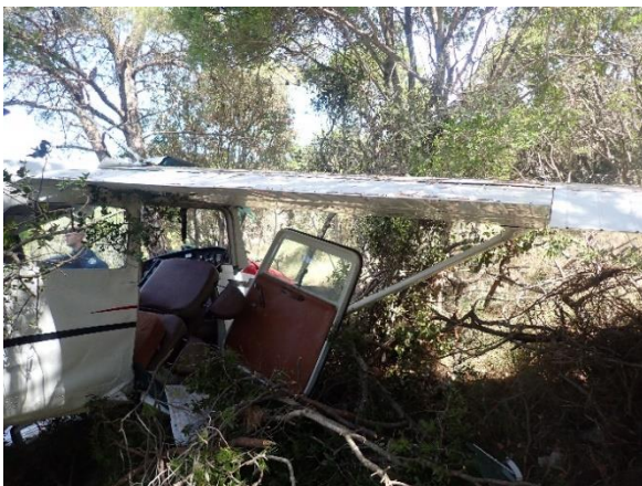
Picture 12 – Retracted right wing flap
