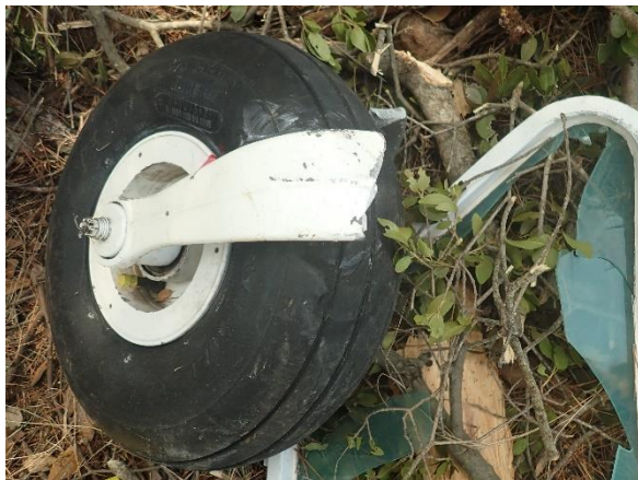
Picture 7 – Broken front landing gear fork
