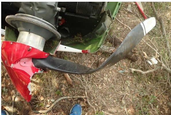
Picture 8 – Bending of propeller arm no. 1
