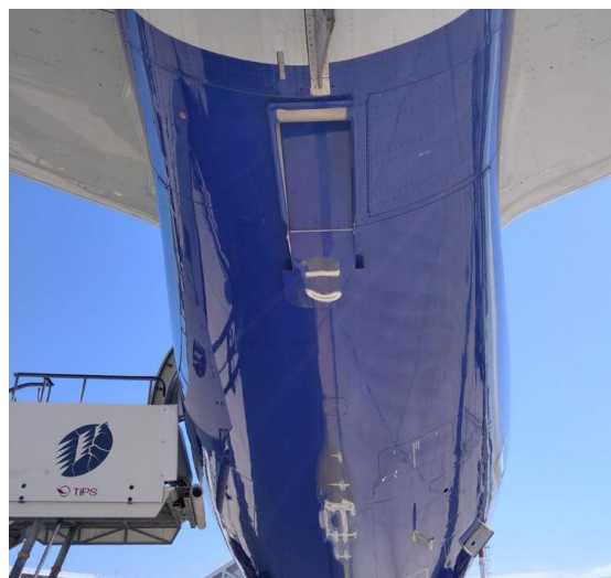
Picture 2 – Skin damage and APU door damage
