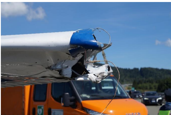
Picture 1 – Damage to the tip of the wing
