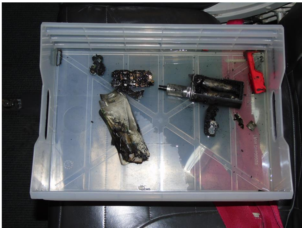
Picture 4 –The electronic evaporator cooled in water after the explosion
