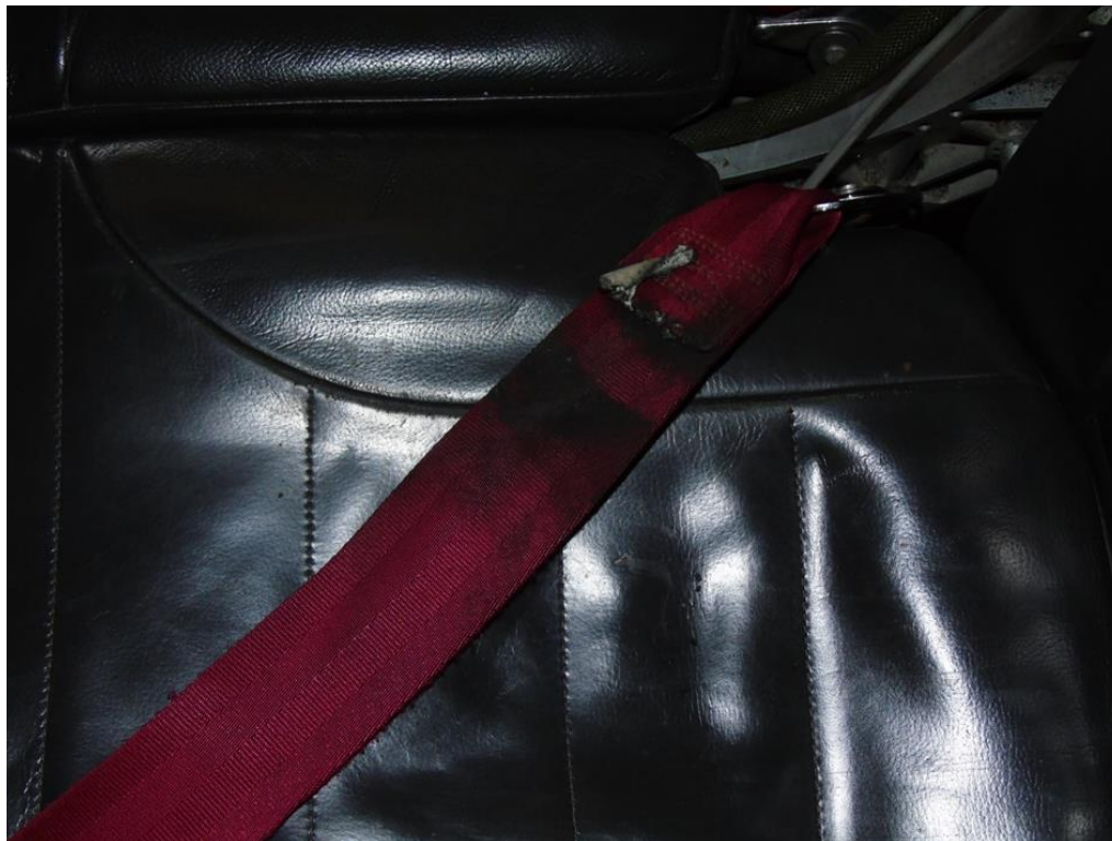
Picture 3 – Burnt passenger seatbelt on the seat no 21D
