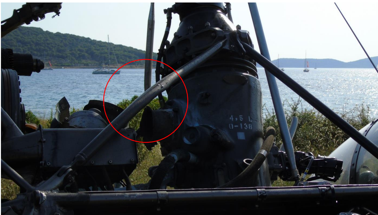
Figure 9 – Bent main gearbox mount
