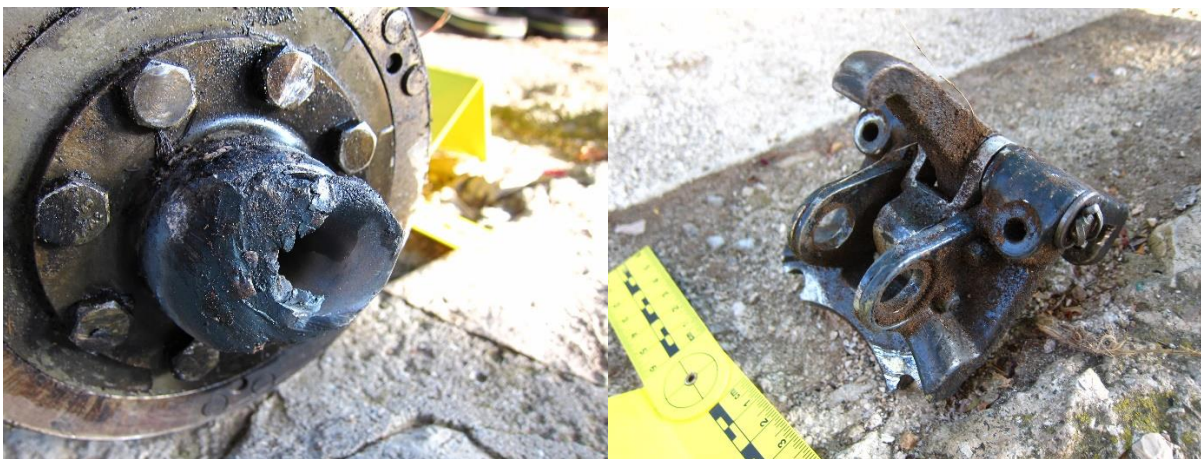
Figure 16 – Point of rupture of input bevel drive shaft Figure 17 – Calliper mechanism
