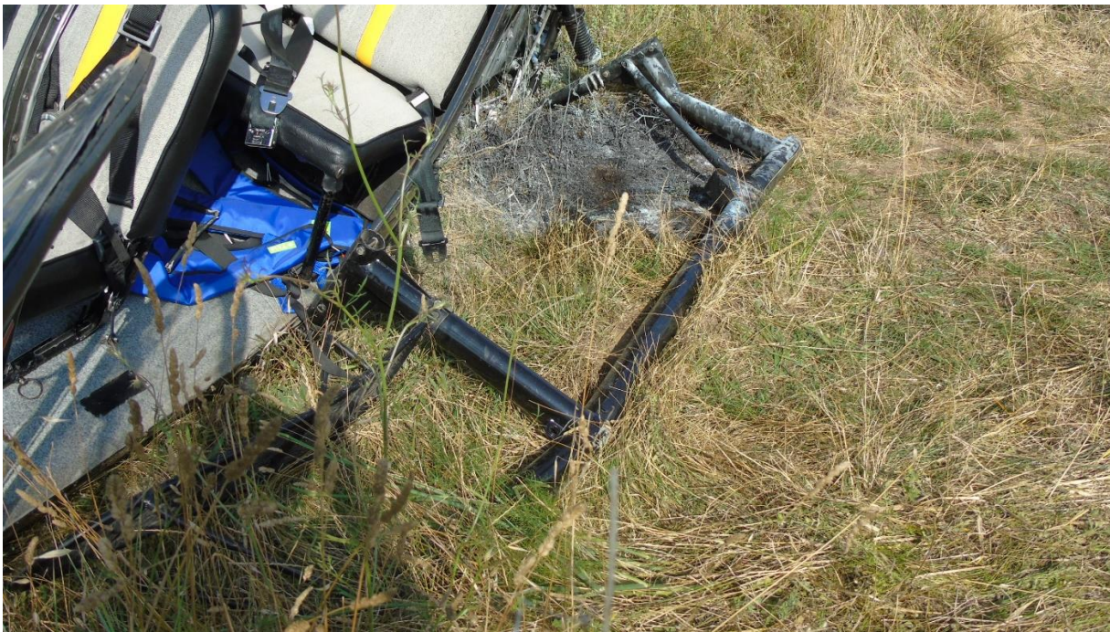
Figure 8 – Bent left skid with the ruptures at the junction points to the helicopter structure
