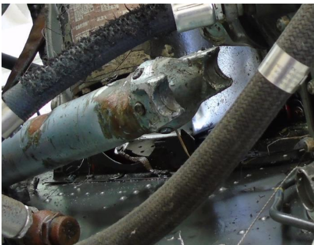
Figure 34 – Cracked cardan shaft universal joint
