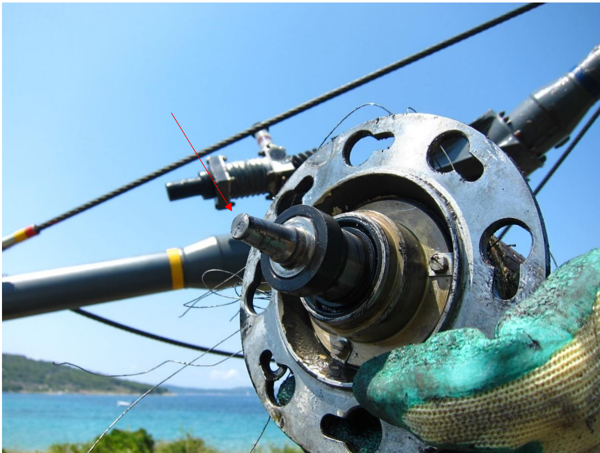
Figure 24 – Broken starter-generator shaft
