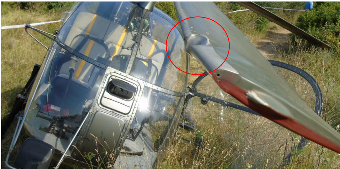
Figure 10 – Damage to the blade no. 1 of the main rotor marked in red
