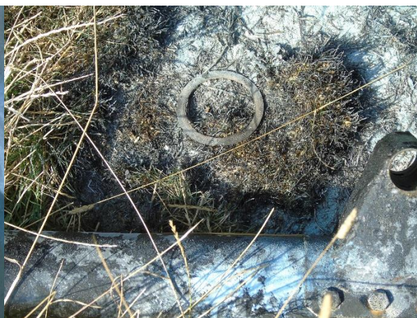
Figure 26 – Seal in the fire site near the skid
