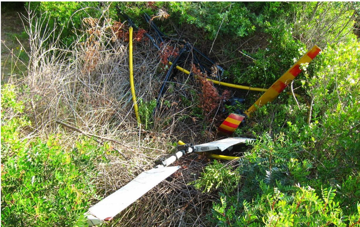
Figure 6 – Part of the separated tail structure with pertaining parts
