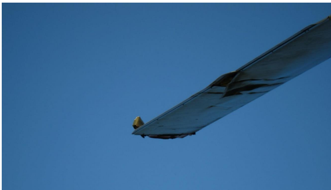
Figure 11 – Damage to the blade no. 2
