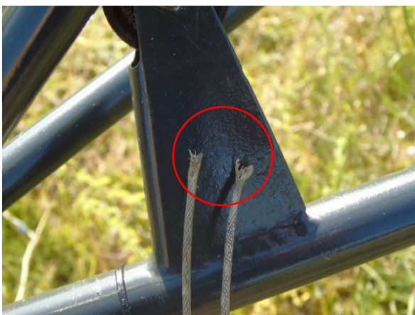
Figure 20 – Damaged tail rotor cable controls
