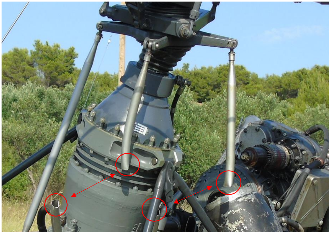
Figure 19 –Cracking points of the two levers for controlling the main rotor blades
