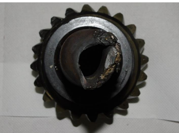
Figure 31 – Point of rupture of the input bevel drive shaft
