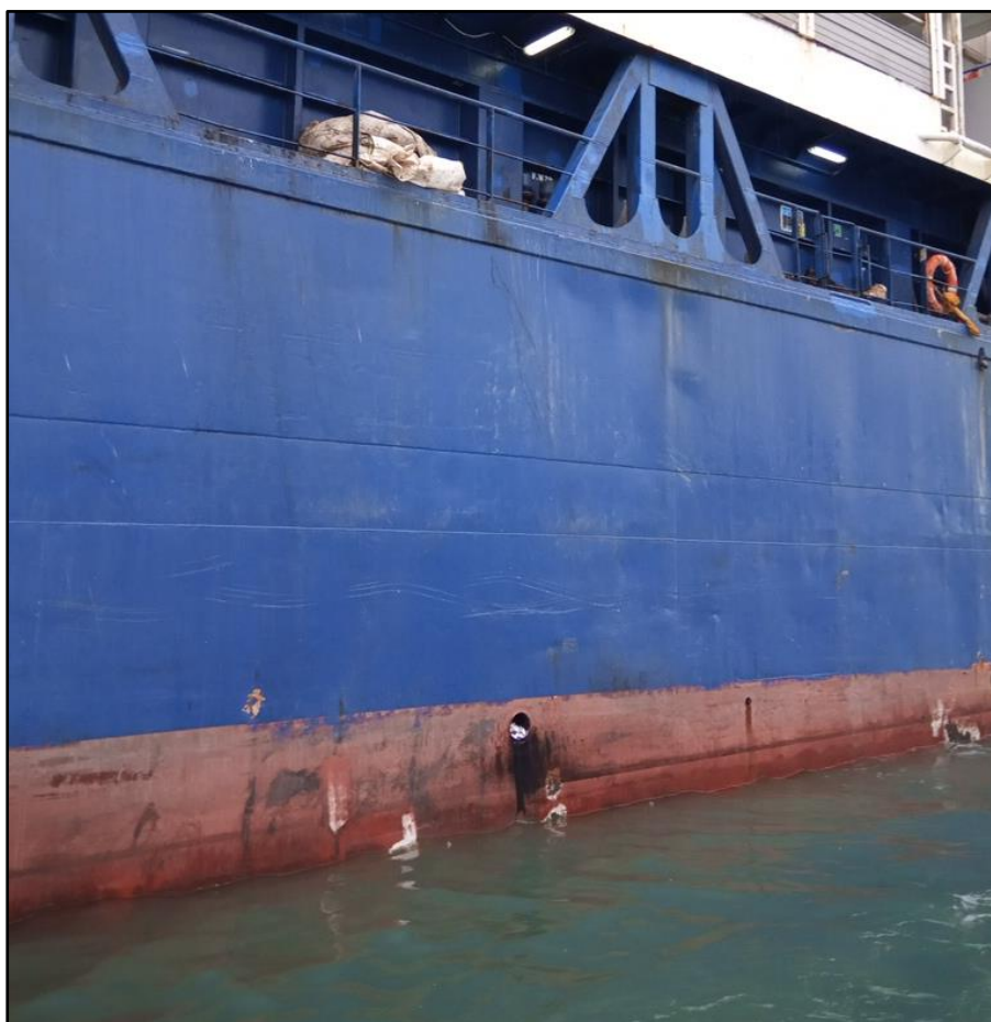
Picture 7 Traces of fuel below the scupper on hull plating of the m/v "Fidelity" (Source: Harbour Master's Office Pula)
