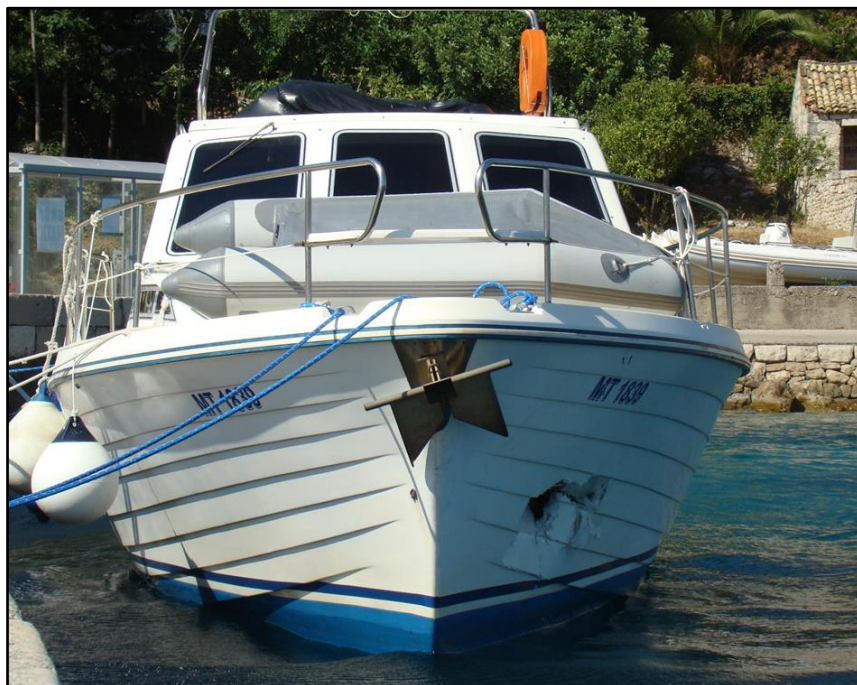
Picture 5 Visible damage to the forward port side of the shell plating above the water level of the boat with registration number "MT 1839" (source: Harbour Master's Office Dubrovnik)
