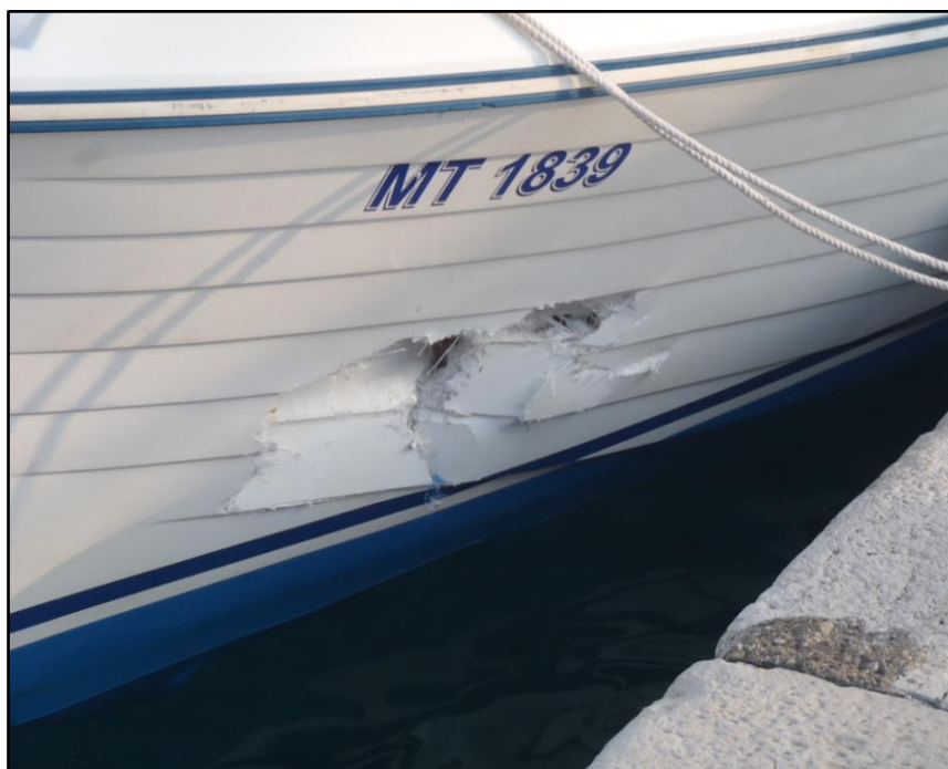
Picture 6 Visible damage to the forward port side of the shell plating above the water level of the boat with registration number "MT 1839"- close up (source: Harbour Master's Office Dubrovnik)
