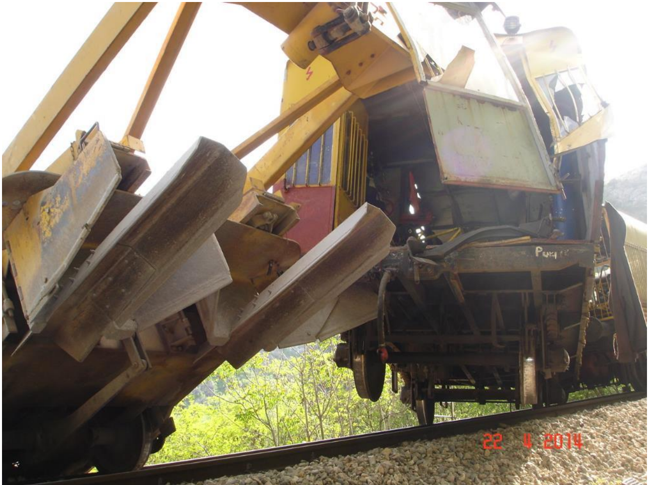
Image 3—the position of derailed vehicles after they stopped (image source: HŽ Infrastruktura d.o.o.)
